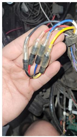
\*Be careful while removing these adapters, will need a small flat head tool to push down the locking clip!!!
