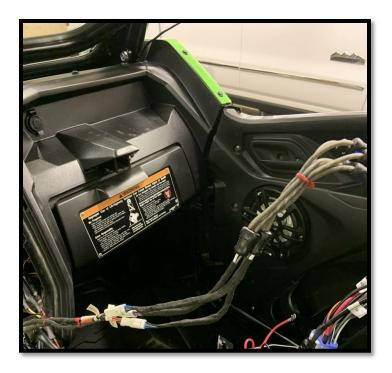
•Plug modular connector that is crimped to the bus bar wiring harness to the modular connector on the back of the head unit.
