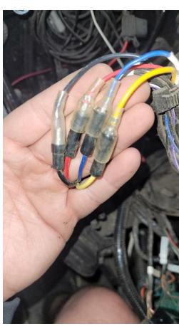
\*Be careful while removing these adapters, will need a small flat head tool to push down the locking clip!!!
